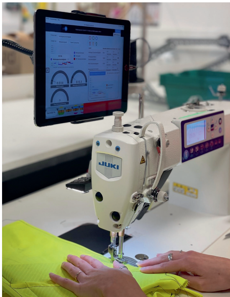
Figure 1: SewGuide intelligent learning assistant reflects real-time data to the apprentice to improve the safety-related sewing process
